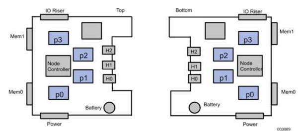
Figure 2-2 shows the location of the processor sockets (along with the processor number) on the processor board.
